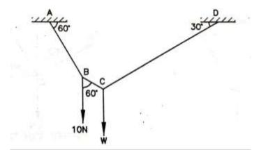
Calculate Tension produced in strings for both the figures as shown below.
