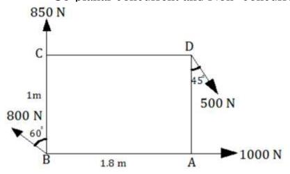
Find the beam reactions of a beam shown in Figure.
