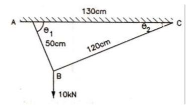
Calculate magnitude and direction of resultant force R of given system of forces using any method.
