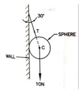
Calculate Tension produced in strings for the figure as shown below.
